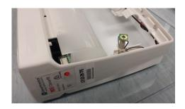
Tamper Sensing Contacts 2 Contacts per Side Cover
